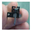
Loosen the screw and remove the lid of electrode. Then replace with a new one. After Cleaning, press the Key 10 times with closing windshield to remove the dust.
