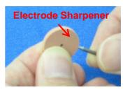
Stick the tip of an electrode into the electrode sharpener and turn/twist the electrode 3-4 times.
